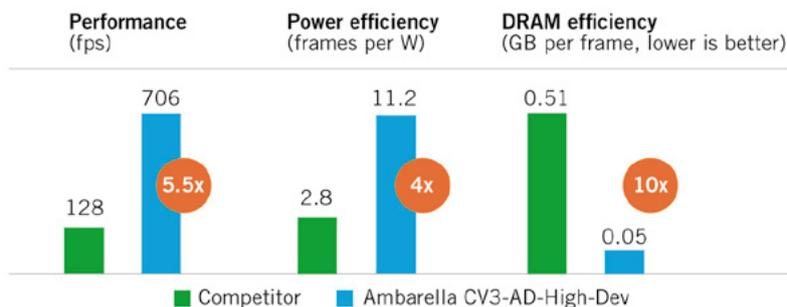
FIGURE 5 Comparison of key performance features of the CV3-AD-High-Dev SoC with similar SoC available on the market (© Continental)
