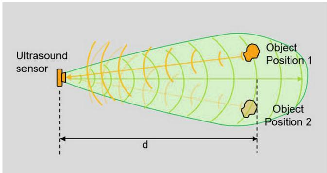
Picture 2: Ambiguity: Ultrasonic sensors can measure the distance to an object by timing the reflection of sound waves, but they cannot determine the object's direction or velocity. The object can therefore be at several different positions in the field of view.
