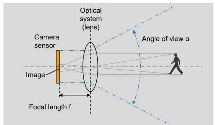
Picture 1: How a digital camera works: The optical system projects an image of the environment onto the sensor. The area covered by the image depends on the focal length and the angle of view.
