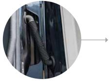
Placement The radar is mounted on the mirror arm at a height of at least 2 meters. 2 Cabling The cables are routed through the door into the cab.
