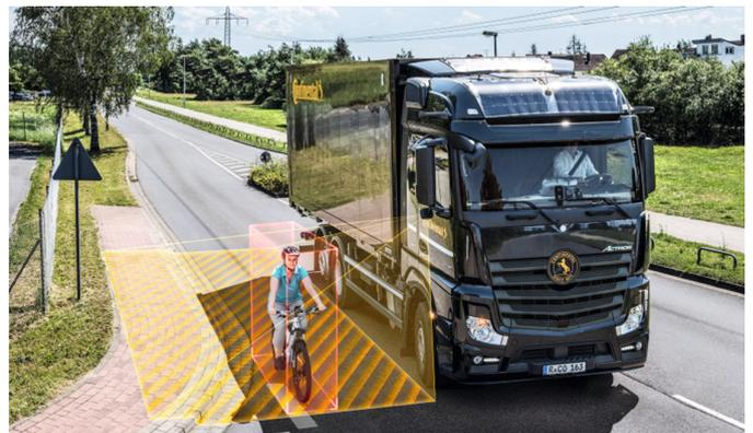
Continental's turn assist uses visual and acoustic signals to warn drivers of a possible collision.
